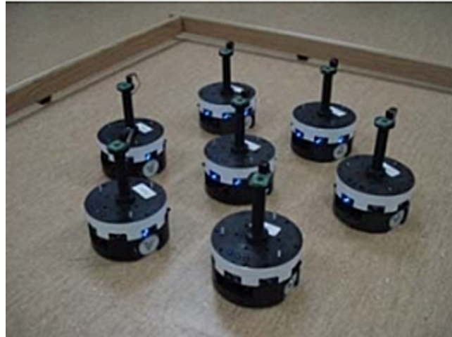
Fig. 44. (Color online) A photo of seven mobile robots (called “Kobots”) moving in a swarm. According to Turgut et al. (2008), the main factor defining the size of the swarm (the number of Kobots flocking together) is the range of communication, and it is highly independent from both the noise (encumbering the sensing systems) and from the number of neighbors each robot had. Source: Adapted from Turgut et al. (2008).
