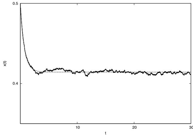
**Figure 9.4** Fraction  $x(t) = n(t)/V$  of unbound A atoms in the chemical reaction  $A + B \rightleftharpoons AB$ . Parameters:  $N = 10^4$ ,  $k_{12} = 0.5$ ,  $V/N \equiv v = 2$ ,  $\omega_{21} = 1$ . The initial condition is  $n_0/V = 0.5$ . The analytical line is the result of the mean-field theory, see exercise 8.6.
