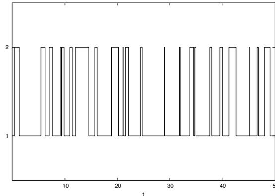
**Figure 9.1** Typical trajectory of a stochastic system that jumps between 2 states using the rates  $\omega_{1 \rightarrow 2} = 0.5$ ,  $\omega_{2 \rightarrow 1} = 1.0$ .
