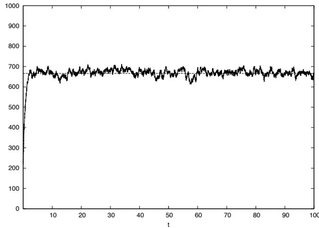
**Figure 9.3** Number of particles in state 1 for an ensemble of  $N = 1000$  particles that can jump between states 1 and 2 with rates  $\omega_{1 \rightarrow 2} = 0.5$ ,  $\omega_{2 \rightarrow 1} = 1.0$ . The horizontal dashed line is the steady state value  $\frac{n_{st}}{N} = \frac{\omega_{2 \rightarrow 1}}{\omega_{1 \rightarrow 2} + \omega_{2 \rightarrow 1}}$ , as found in (8.11).
