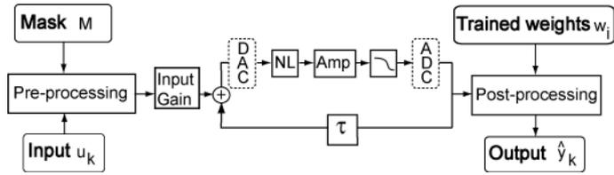
**Supplementary Figure S7: Schematic representation of the experiment** The Mackey Glass system is realised by a nonlinearity (NL), and amplifier (Amp), a low pass filter, and a delay. DAC and ADC, Digital to Analog Converter and Analog to Digital Converter respectively. The input gain block corresponds the parameter  $\gamma$ , while the amplification block corresponds to  $\eta$ .
