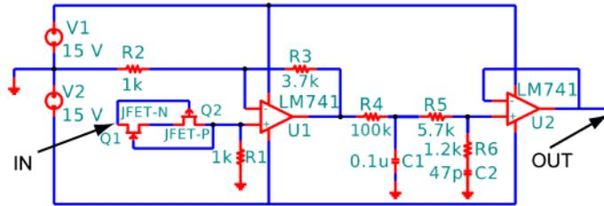
**Supplementary Figure S8: Schematic representation of the hardware node** Two FET transistors, one n-channel (Fairchild 2N5457) and one p-channel (Fairchild 2N5460) generate the nonlinear function itself. An amplifier (LM741) provides the desired magnification factor and two RC-circuits allow to set the time constant of the circuit.  $R1 = 507\Omega$ ,  $R2 = 1k\Omega$ ,  $R3 = 3.7k\Omega$ ,  $R4 = 100k\Omega$ ,  $R5 = 5.7k\Omega$ ,  $R6 = 1.2k\Omega$ ,  $C1 = 0.1\mu F$ ,  $C2 = 47pF$ .
