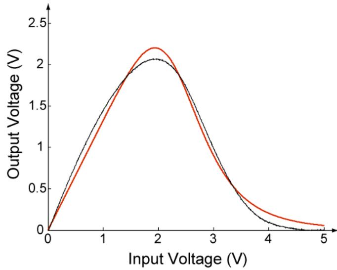
**Supplementary Figure S9: Fitting of experimental transfer function** Experimental transfer function (black) compared to a fit using the Mackey-Glass equation (red). Fit parameters correspond to  $C = 1.33$ ,  $b = 0.4$  and  $p = 6.88$  (eq. S20).
