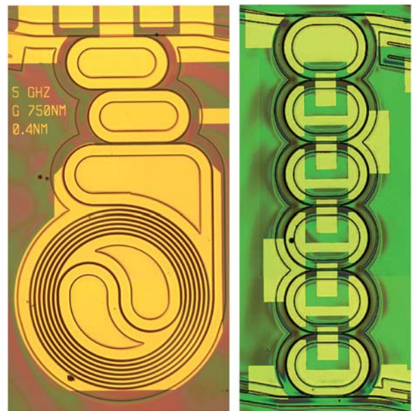
FIG. 50 (color online). Left panel: Chip of semiconductor ring lasers, emitting at \lambda = 1.55 \mu\text{m} . The top ring is connected to a bus waveguide and the bottom ring to a spiral, implementing delayed feedback. Right panel: Chip of six coupled ring lasers (cavity length 1250 \mu\text{m} ), illustrating the integration perspectives for coupled lasers. Courtesy of Marc Sorel, University of Glasgow.
