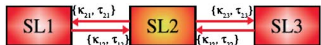
FIG. 23 (color online). Chain of three mutually coupled semiconductor lasers interacting bidirectionally with a time delay.
