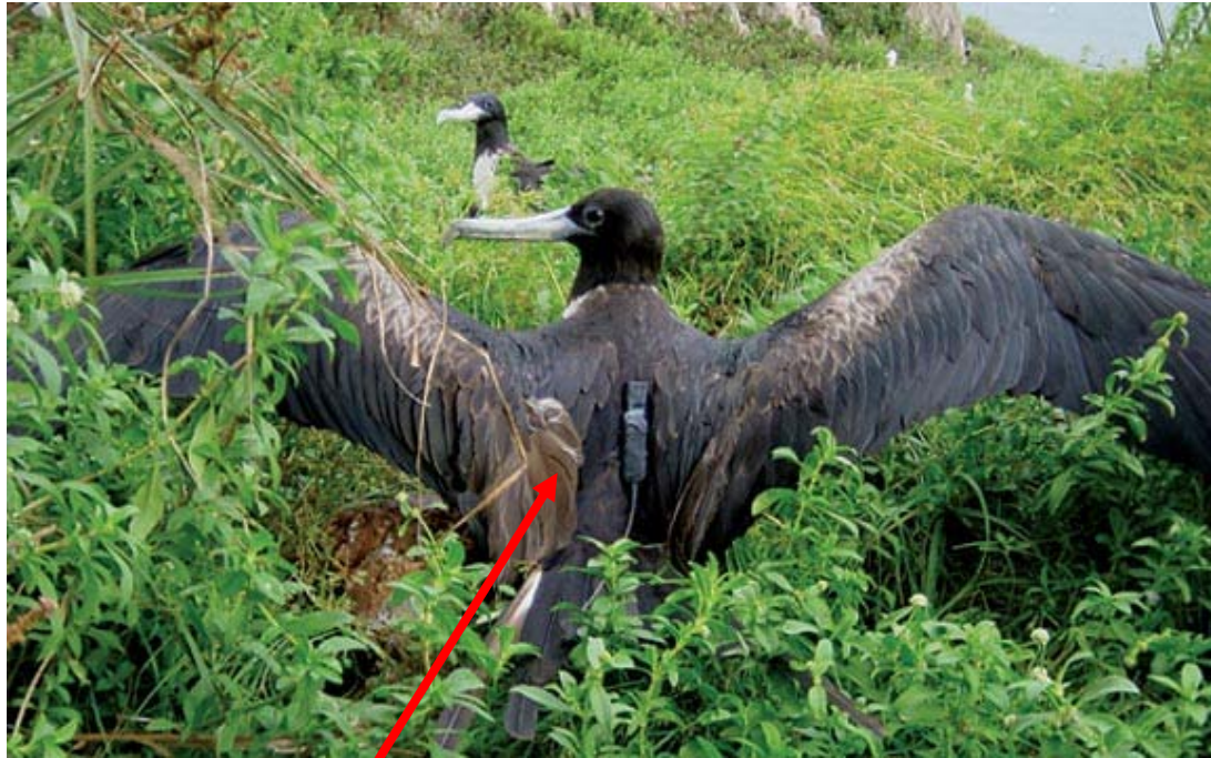
Satellite transmitter and altimeter (total weight : 1 to 3% mass of adults, max 45g)
