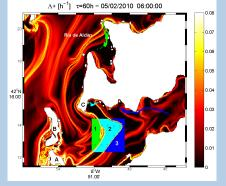
Instantaneous FTLE field in the Ria de Vigo computed from trajectories of arificial fluid particles in the model surface flow. Different water masses (1.2.3) are defined between sharp ridges of the FTLE field, corresponding to distinct final positions of the particles.
