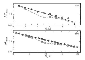
FIG. 3. AC peak (gray squares) and its envelope (black crosses) around the delay time vs the number of elements in the ring for (a) semiconductor lasers and (b) Ikeda oscillators. An exponential fit,  $\alpha \exp[-\beta(N-1)]$ , has been calculated of the envelope (solid black lines). Black circles indicate the maximum of the envelope of the AC peak at  $t=M\tau$  (t=MT) of one laser (Ikeda) with delayed feedback. The gray dashed lines are guides to the eyes.
