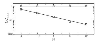
FIG. 4. Maximum value of the cross correlation (CC<sub>max</sub>) between the sender (SL N/2) and the transmitter (SL 0) (black squares) and between the sender and receiver (SL N/2) (gray circles) vs the number N. The solid black line is an exponential fit using  $\alpha \exp[-\beta(N-1)]$ . The gray line is a guide to the eyes.
