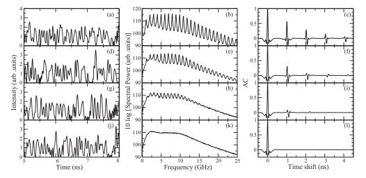
FIG. 2. Time traces (left panel), power spectra (middle panel), and normalized intensity autocorrelation functions (AC, right panel) of the emission of one laser for different values of N. (a)–(c) correspond to a SL with delayed optical feedback, (d)–(f) to two bidirectionally coupled SLs, (g)–(i) to 4 SLs in a ring configuration, and (j)–(l) to 100 SL in a ring configuration.
