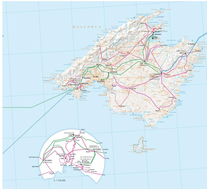
Figure 1: Mallorca's power grid. Green lines are 220 kV transmission lines, blue lines are 132 kV transmission lines and red lines are 66 kV transmission lines.
