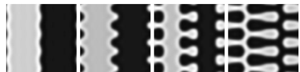
FIG. 6. Transverse modulational instability for a flat domain wall. E_0 = 1.4 . Snapshots at times t=0, 400, 600, and 860 .
