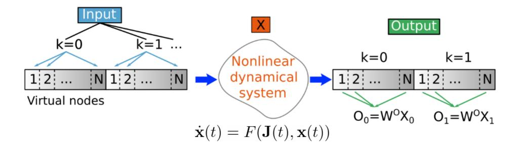
Time-multiplexed input with random scaling allocated to different temporal slots
