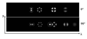
FIG. 8. A numerical snapshot picture of the spectrally resolved near-field intensity distributions of the VCSEL without FSF, for I=4.5 mA.
