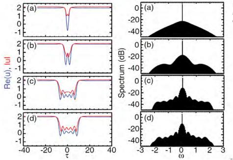
**Figure.** Temporal profiles (left) and spectral intensities (right) of dark pulse KFC.
