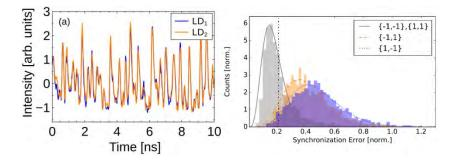
Figure. (Left) Time series demonstrating high quality synchronization. (Right) Experimental synchronization error, in which the gray histogram (and correspondingly fitted curve) represents the matched bits while the other two represent the mismatched bits of different sign
