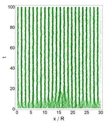
Trajectories of repelling particles forming a cluster crystal in one spatial dimension. Space is in the horizontal, and time in the vertical.
